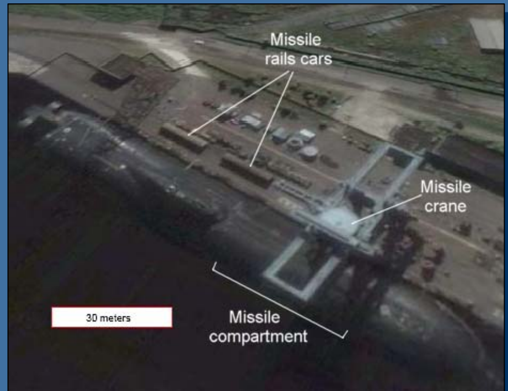
Typhoon-class SSBN loading or offloading missiles at Severodvinsk naval base, 2005. Image: GoogleEarth
