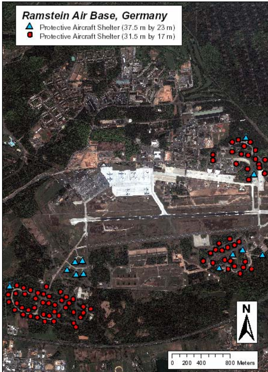
Ramstein Air Base, Germany (May 8, 2003): This base is located in southern Germany (49°26'N, 07°36'E) south of Mannheim. There are 90 Protective Aircraft Shelters (PAS) on the base, 12 of which are the large version (37.5x23 meters) and 78 the smaller shelters (31.5x17 meters). Fifty-five of the shelters are equipped with WS3 Vaults for nuclear weapons storage with a capacity of 220. The vaults were completed in 1992. Up to 130 B61 nuclear bombs are stored at the base, depending on the status of the weapons removed from Memmingen Air Base and Araxos Air Base. Of these, up to 90 bombs are for delivery by U.S. F-16C/Ds of the 22 nd and 23 rd fighter squadrons of the 52 nd Fighter Wing based at the nearby Spangdahlem Air Base. Up to 40 of the bombs are for delivery by German Air Force PA-200 Tornados. Source: DigitalGlobe.
