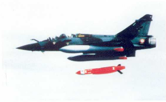
APACHE Cruise Missile Dropped from a Mirage 2000 Aircraft
