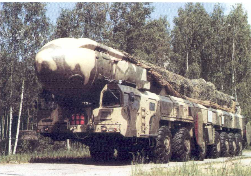
The Russian SS-25 missile is launched from a canister carried on a seven-axle transporter-erector-launcher.
