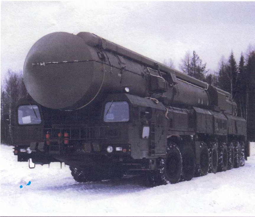
Russia's road-mobile SS-27 is carried in a canister on a new eight-axle transporter-erector-launcher.
