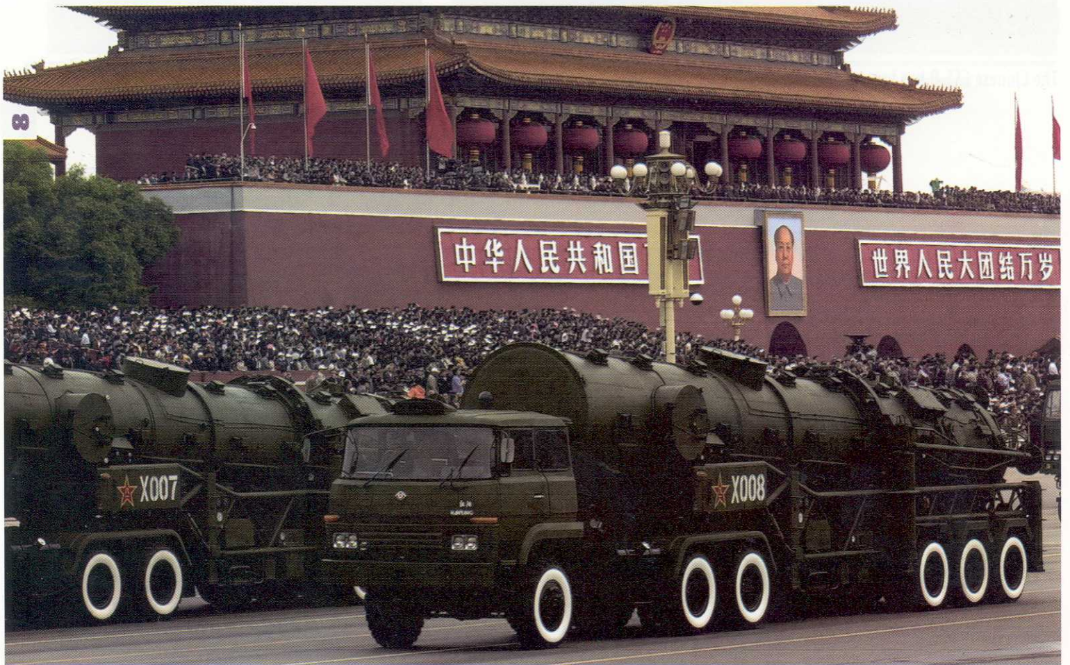
The Chinese CSS-5 is a two-stage, solid-propellant MRBM capable of reaching targets in the Pacific Theater and most of Asia. The missile is in a canister on a towed erector-launcher.
