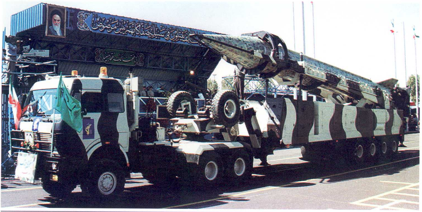
The Iranian Shahab 3 is a single-stage, liquid-propellant missile based on the North Korean No Dong MRBM.
